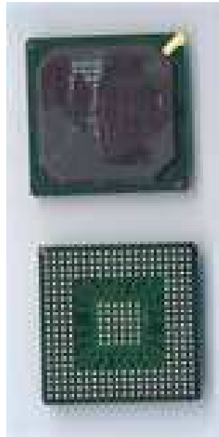
BGA=Ball Grid Array
